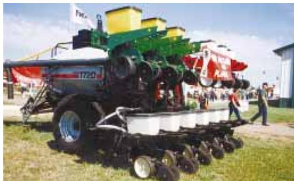
Flexicoil unit shown has Deere and Kinze row units mounted on a 30-ft. folding toolbar that's 3-pt. mounted to a 130-bu. tank.
