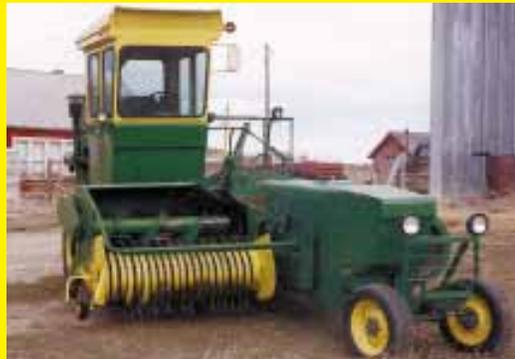
type baler it was so hard to see that there might be four or five broken bales before we'd notice. I mounted extra lights on this machine which helps a lot.
