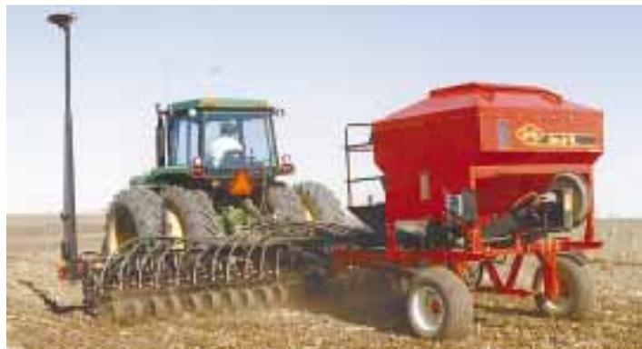
Gandy's air seeding system features Acra-Plant notched, double-disc openers mounted on a 7-in. sq. toolbar. Shown is a 15-ft. toolbar model with a 64-bu. tow cart.
