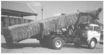
Rig loads seven 3 by 4 by 8-ft. bales weighing up to 2,000 lbs. apiece. It can travel up to 40 mph in the field and 55 mph down the road.
