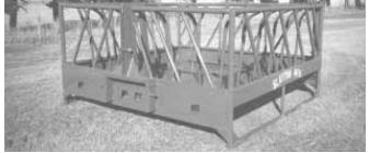
Bale feeder is equipped with a rear gate that swings open for easy loading.
