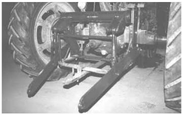
Add-on 3-pt. bolts onto existing drawbar and is raised and lowered by a single 3 by 6in. hydraulic cylinder, with a second cylinder optional.
