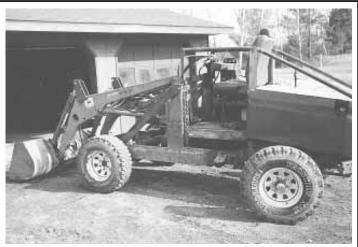
"The loader didn't have cylinders on it when I bought it so I added 3-ft. long cylinders and built brackets for them. To steer I simply move a lever back and forth. I use a two-way spool valve to operate the loader and bucket. The hydraulic pump off an old Deere combine provides power steering. The pump originally was connected to cables that controlled the combine's steering system. I connected the cables to the Blazer's steering system."
