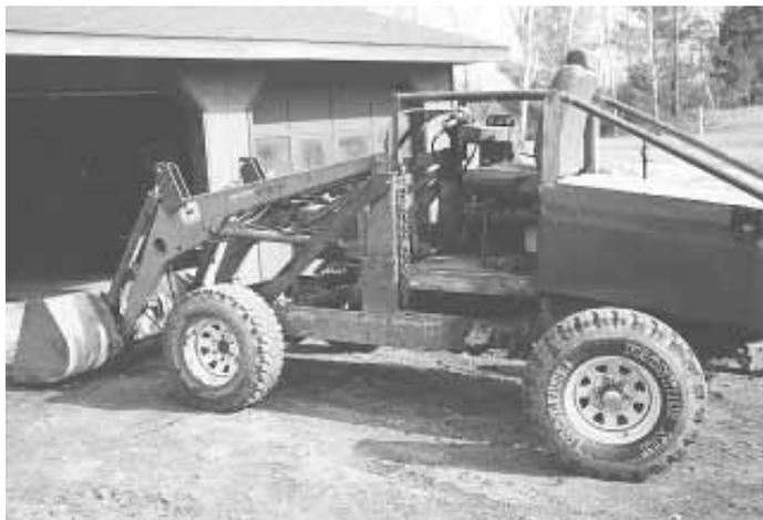
"The loader didn't have cylinders on it when I bought it so I added 3-ft. long cylinders and built brackets for them. To steer I simply move a lever back and forth. I use a two-way spool valve to operate the loader and bucket. The hydraulic pump off an old Deere combine provides power steering. The pump
