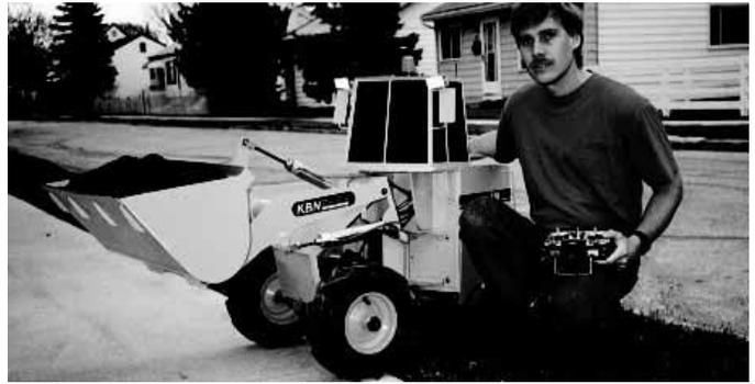
Nolman operates mini payloader with a commercial model airplane radio control unit.
