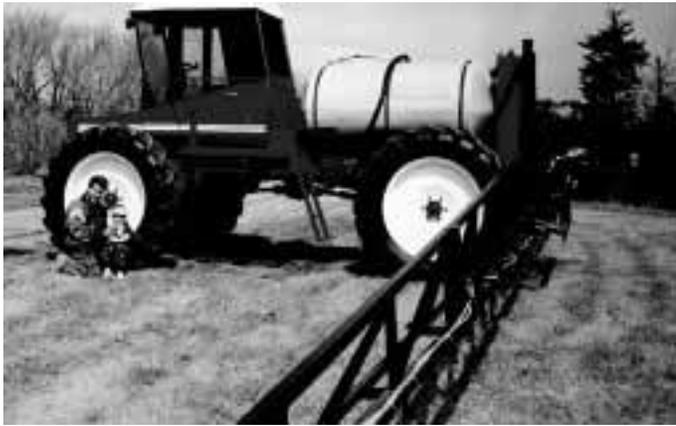
The Delorme's used the frame and axles from a 6-WD Army truck to build the sprayer and equipped it with a 550-gal. tank and 88-ft. boom. The cab is off a Hesston haybine.
