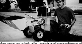
Nolman operates mini payloader with a commercial model airplane radio control unit.
