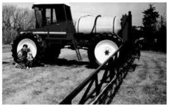
The Delorme's used the frame and axles from a 6-WD Army truck to build the sprayer and equipped it with a 550-gal. tank and 88-ft. boom. The cab is off a Hesston haybine.
