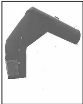
**Kit adds 1 1/2 to 4 1/2 ft. to length of down spout on combine unloading auger.**
