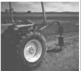
Wire roller's 20-in. dia. spool has a 2-in. dia. shaft that mounts in place of auger bit on Bush Hog post hole digger.
