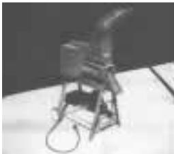
the machine. On the opposite side, there's a steel wheel and rod arm that rotates a piston made of 2-in. sq. tubing fitted with a catch on back to hold the cans, which enter the machine through a rack. Ears welded on each side of the machine keep cans in alignment. Cans are contained in a 6-in. long compression chamber, where they're crushed down to 3/4-in. thick. The crusher is built on an angle iron frame and mounts on two wheels so it's portable.
