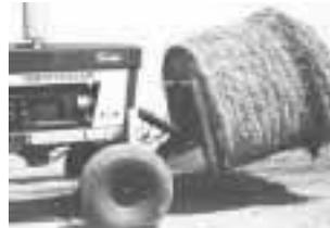
blade and frame off when we're not using it, I decided to leave the mounting bracket on our Farmall 1466 all the time. The bracket reminded me of a 3-pt. hitch so I took two 10-in. lengths of 3/4-in. thick, 3 1/4-in. wide strap iron we had and bolted them to the frame through existing slots near the bottom of the hydraulic cylinder arms. They serve as two members of a 3 pt. hitch for our commercial bale carrier, which we secure at top with a chain that serves as a third member.
