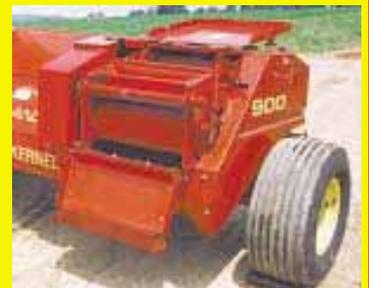
Kit consists of two 8 1/2-in. dia. by 22-in. long steel rollers with 1/4-in. machined grooves. Rollers turn at different speeds to provide a shearing action that results in better breakage of kernels.
