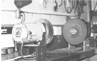
an arbor and washers to the threaded end of the shaft so you can fit a grinding wheel or abrasive wheel on the end."
