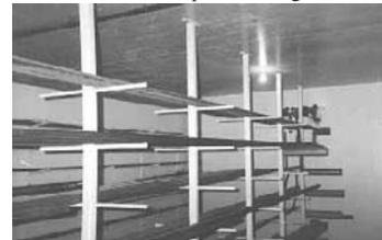
angle iron neat and organized in our shop. A series of steel pipes runs from ceiling to floor with 16-in. long steel rods welded onto each side of the pipes.
