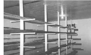
angle iron neat and organized in our shop. A series of steel pipes runs from ceiling to floor with 16-in. long steel rods welded onto each side of the pipes.
