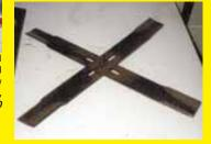
I made "cross blades" for my push-type mower that goes right through brush with ease. The cross blade consists of two 22-in. blades that are overlapped, squared up, and holted in place
