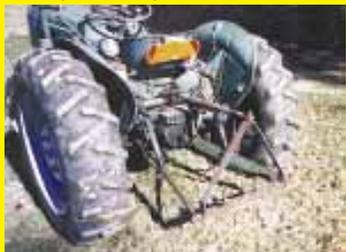
It's simply a section of 1/4 by 2-in. steel bent into an A-shape and welded to the ends of the drawbar. There's a hole in the apex to accommodate the top link and pin, which keeps the drawbar from rotating and, in fact, keeps it level at any hitch height.
