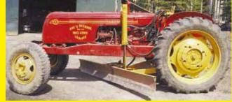
Here's a 1948 Cockshutt model 30 row crop tractor that I modified to handle a "mini" grader blade I built to grade roads and push snow.
