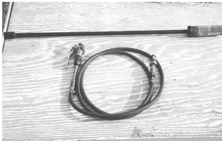
Put together for about $20, the burner produces a flame 2 ft. long and 12 in. in dia.
