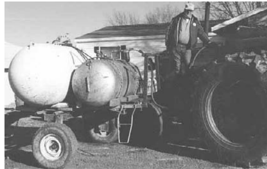
Roth uses his anhydrous tank pressure washer to clean off radiators in the field and his anhydrous tank fuel carrier to keep two tractors going for two or three days.
