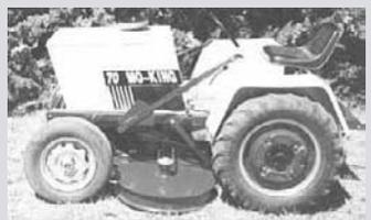
Kuhn's mower is powered by a 4-cyl. engine out of a Toyota car.
