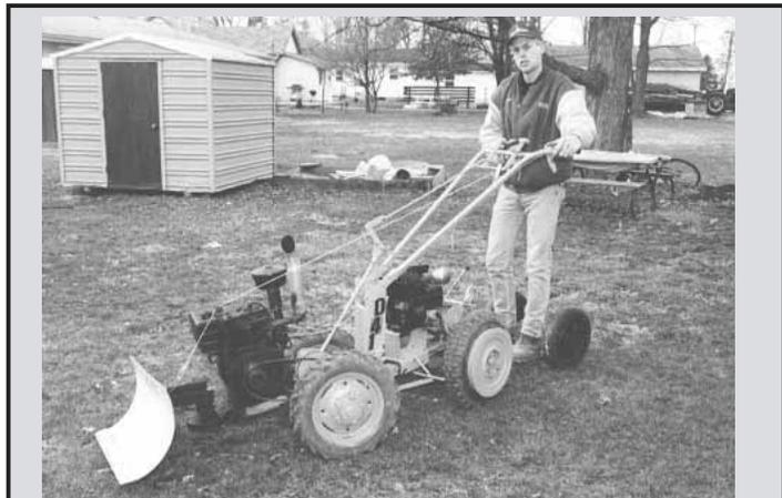
Garden tractor is powered by a 10 hp Briggs & Stratton engine up front and a 5 hp Briggs & Stratton engine in back.
