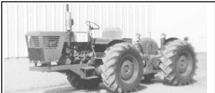
To join the rear ends, Moshondz built a hinged frame out of 3-in. angle iron.
