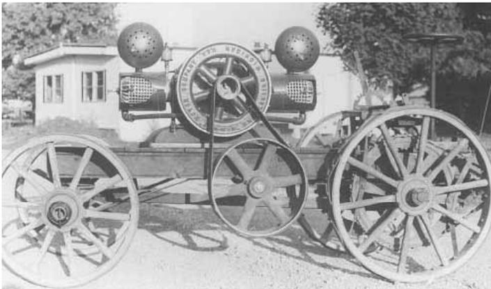
Henkel's all-pine tractor was used in the early 1900's to belt-drive corn grinders, water pumps, and other equipment.
