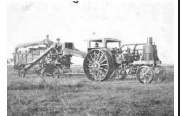
Hausler created an early combine by hitching a stationary threshing machine and a push binder to an Avery tractor.
