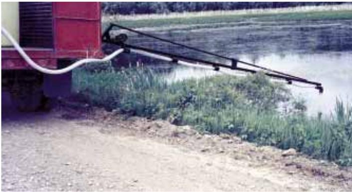
The 21-ft. long boom mounts on back of Berberat's 1-ton truck and is hinged, allowing it to pivot 180 degrees and pull clean water out of ditches or streams.
