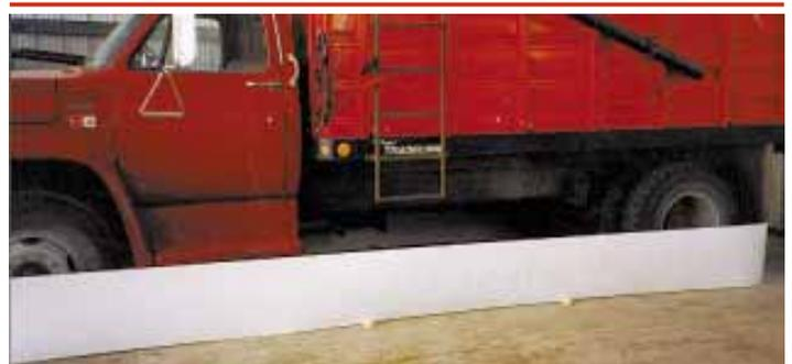
An 18-in. high wall of rigid plastic encircles each piece of equipment, keeping mice out. Eliminates the need for poisons and traps.
