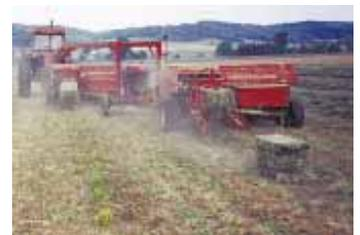
Axle at back of hitch is designed to run at a slight angle. Engine hydraulically pivots to stay in line with baler's pto shaft when turning at end of field.
