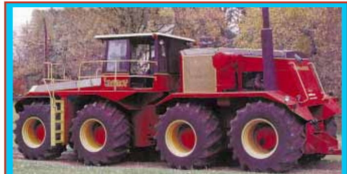
In field tests, the 600 hp “Big Roy” easily handled a 118-ft. wide cultivator at up to 6 1/2 mph and a 20-bottom plow pulled 12 in. deep.
