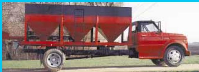
Stienessen mounted 3-hopper bulk seed handler on his Chevy C-50 2-ton truck. A brush auger runs under the three hoppers to back of truck, where a second brush auger can be swung out and up for filling planters and drills.
