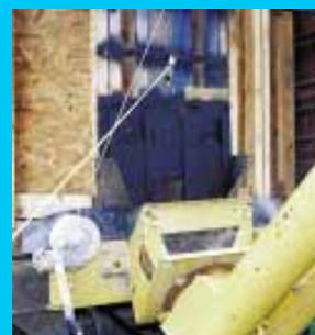
Compartments empty out through sliding gates at back of truck. A rope and pulley are used to lift each gate.
