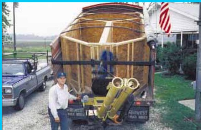
Removable wooden box is fitted with 3 compartments to handle different soybean varieties in Thoele's 2-ton truck. A 14-ft. drill-fill auger mounts on back.
