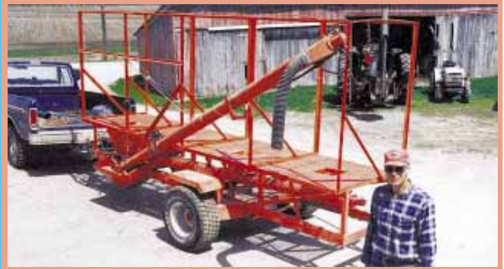
Caddy handles four 2,000-lb. bulk bags. David and Paul Hartweg built the 16-ft. long caddy on an old Artsway 425 grinder chassis equipped with weigh bars.
