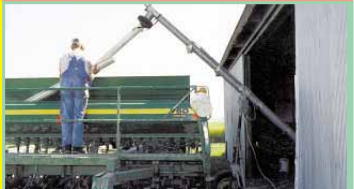
Ruppert attached an old lawn mower tire between auger downspout and a 4-in. dia. PVC pipe. Tire flexes enough to allow pipe to swivel up to 45 degrees in any direction.
