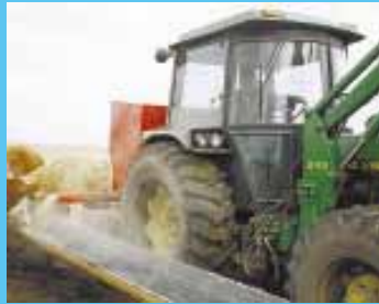
Grain flow is hydraulically controlled from tractor cab.
