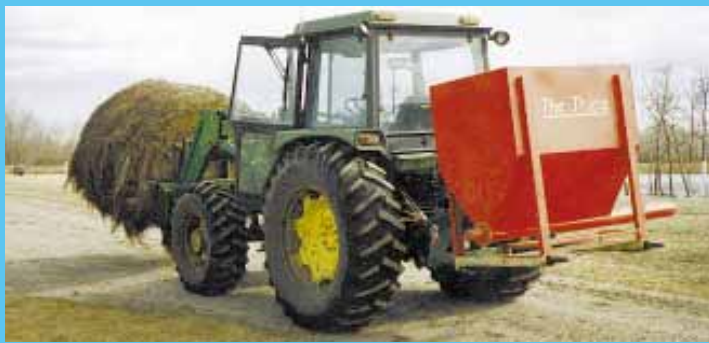
The 3-pt. mounted hopper uses a 5-in. dia. drill fill auger at the bottom to deliver feed to Flaman's cattle. Hopper holds 40 bu. and mounts on feet made of 3-in. sq. tubing.
