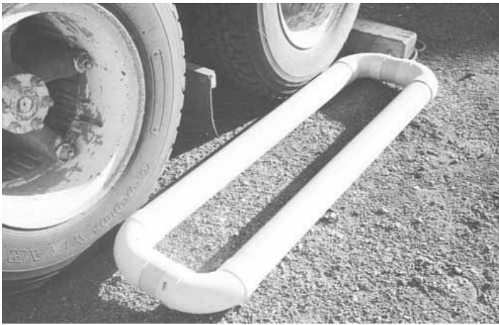
“Back-up guide” is made from 10 ft. of 4-in. dia. white PVC pipe, making it as easy to see at night as it is in broad daylight.
