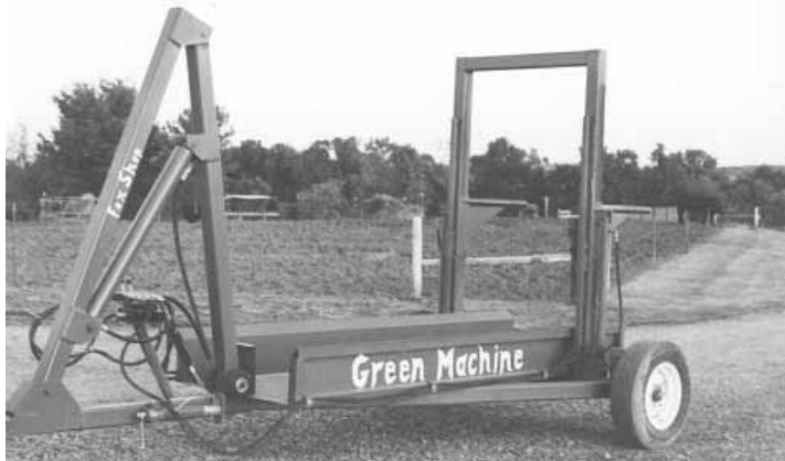
Bale pusher on front is powered by a 36-in. long, 3 1/2-in. dia. hydraulic cylinder.
