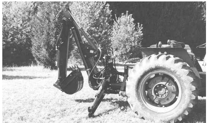
Backhoe features a 12-ft. reach, compared with 8 to 10-ft. reach available on most commercial models.
