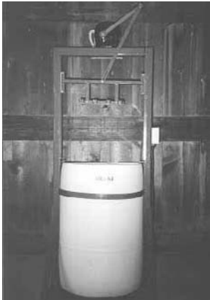
Scalder stands 82 in. high and is powered by 8 rpm gear motor on top.
