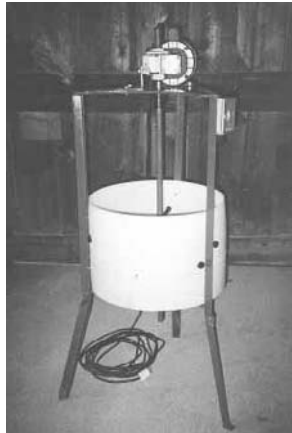
A wheel inside is fitted with rubber fingers that "pluck" chickens.
