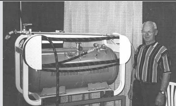
"Gophinator" consists of a 25-gal. anhydrous tank mounted on a frame and fitted with 50 ft. of hose.
