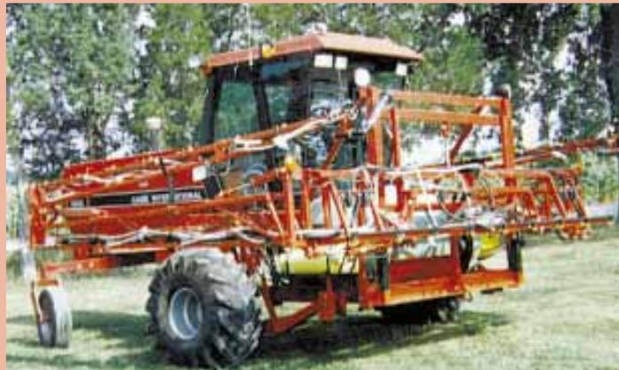
Hydraulic fold boom folds back against the sides of the swather for transport. With its
