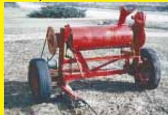
I stripped the baler down to the large power drum. Then I cut around the ends, close to the drum, leaving the ends on the shaft that goes through the drum. Then I removed the drum. Next I welded 1/4-in. chains to the shaft, spacing the chains about 4 in. apart. The chains are spiraled around the shaft to make a sort of auger. The chains were just long enough to barely touch the outside of the drum after it was reinstalled.
