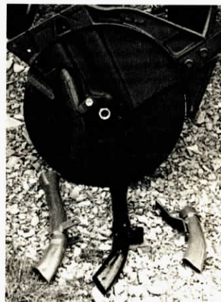
Add-on seed tubes drop seed directly into furrow between disc openers.
