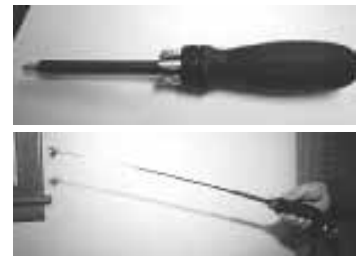
When magnet is retracted, a screwdriver bit can be inserted into the end of the tube (above). It extends out to 14 in. (below).
