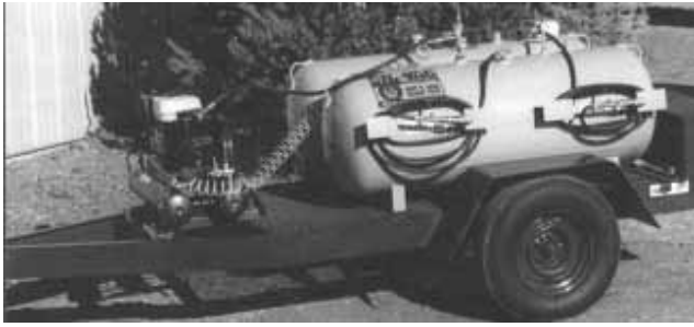
"Oil Vac" is equipped with twin 125-gal. tanks and an compressor on front.
