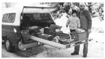
Brian R. Hebden, Springville, N.Y.: "I have easy access to my tools thanks to this pull-out tool tray which I built into the back of my pickup. The tray slides in and out of the bed. I used 2 by 4's and a sheet of 4 by 8-ft. plywood to make the tray. Garage door hangers and caster wheels underneath the tray
