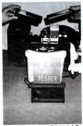
Portable freezer reduced untreated diesel fuel on left to solid mass of jelly; treated fuel on right was still flowable at 40° below zero.
