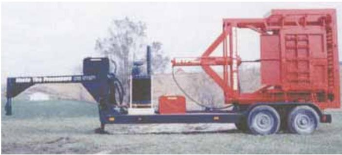
Waste Tire Processors feeds whole scrap tires into its home-built baler, which compresses them and uses galvanized 9 ga. wire to hold them together.
