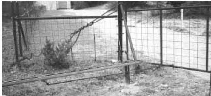
Opener pushes and pulls on a 10-ft. rod to open and close gate.
