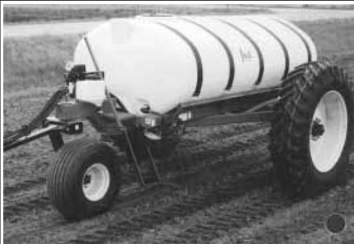
Big tires provide flotation and roadability, while the sprayer's low profile allows you to see the equipment you're pulling.
