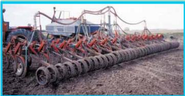
Steffen mounted a series of 15-in. spare tires on back of his Friggstad 41-ft, air seeder. Tires mount in seven sections and are spaced 1 ft. apart.
