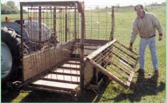
Back side of spreader is hinged, allowing it to be folded down for loading bales. Spreader's unloading apron is driven by a hydraulic motor.
