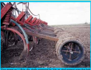
Tires mount on 1 1/8-in. dia. shafts supported by 3-in. sq. steel support arms that bolt to back of air seeder. Down pressure is applied to each section by a pair of coil springs mounted at top of each support.
