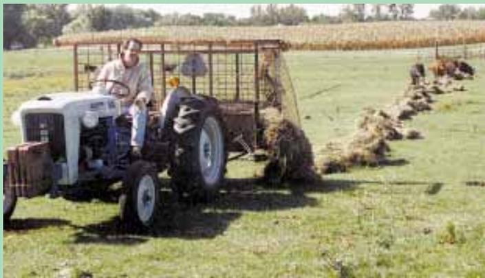
Deere ground-driven spreader was converted into a pto-powered, 3-pt. mounted feeder. A steel frame built under the spreader holds it sideways across back of tractor.
