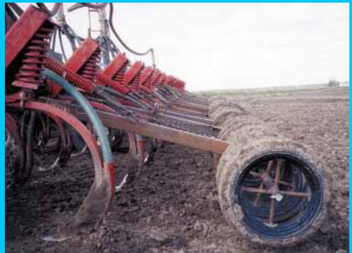
Tires mount on 1 1/8-in. dia. shafts supported by 3-in. sq. steel support arms that bolt to back of air seeder. Down pressure is applied to each section by a pair of coil springs mounted at top of each support.
