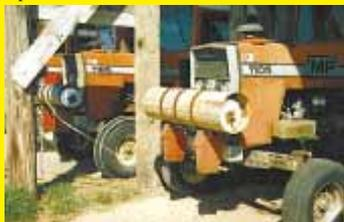
in the center of the other. We've mounted them on six of our Massey 1105 tractors with brackets made of chain and pipe that attach to the hand holds of the tractors' suitcase weights.
