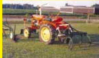
system from 6 to 12 volts and built and installed a 3-pt hitch and hydraulic lift from an electric/hydraulic unit from a 2 1/2-ton truck tailgate lift. I built a one-row crop cultivator and front lift from a front blade from a 4-row cultivator. I also built a 3-pt. single bottom turn plow from a 1-pt. Cub Farmall turn plow. I installed a pto and pulley off an old Avery frame and rear end I bought.
