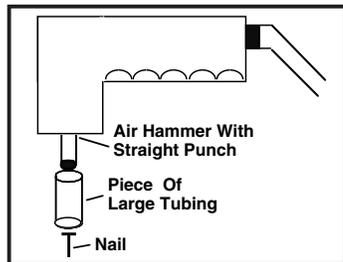
tubing a little larger in dia. than the 7/8-in. dia. straight punch attachment and a little longer than the nails you're driving. Slip this 'guide' over the nail and hammer away. The punch will never slip off the nail head, as it would without the guide, and nails go in effortlessly. It even works to drive bent box nails or 12-in. spikes. If I am working on a large project, I start a bunch of nails, then come back and run them all in with the air hammer. I use a Snap-On model 50 air hammer."
