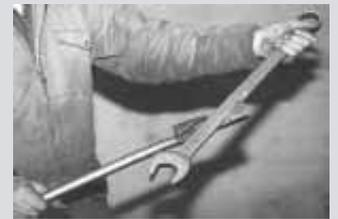
**Tool has an angled slot that "wraps around" the arm of an open-end wrench, providing additional leverage.** market the tool.
