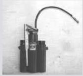
"Caddy" holds two tubes of grease and a gun and can be mounted in the shop or on a tractor, combine, or other equipment.
