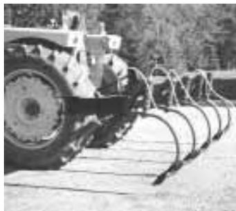
Parker built his own 5-row sidedress unit using a toolbar off an anhydrous applicator and shanks off a chisel plow. Shanks are fitted with liquid fertilizer knives.
