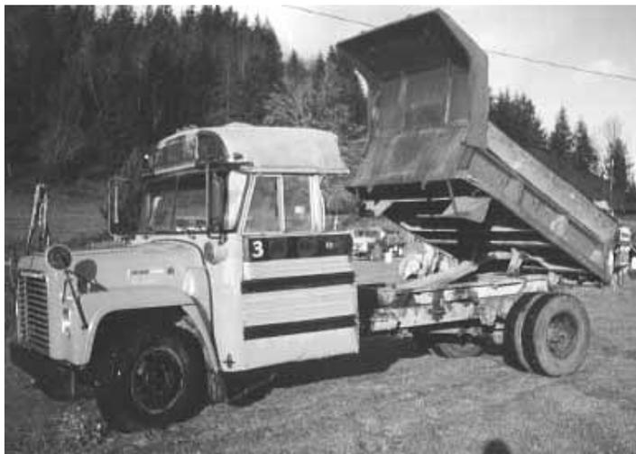
Sassmen stripped bus down to the frame from the driver's seat back, then shortened the frame by 13 ft. and retained the bus's original rear axle and tires. Box is dumped by a pto-driven hydraulic pump off the truck's transmission.
