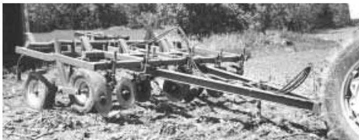
He converted a Deere 1610 13-shank (15-in.) chisel plow to wider spacings for better trash clearance. He removed six of the shanks and respaced the remaining seven on 22 in. spacings. He also added seven Yetter high residue coulters on front of toolbar.
