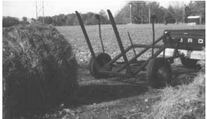
Two-wheel caddy carries bale on a rectangular steel cradle equipped with two forks at bottom and a removable spear in middle. It can be pulled behind a pickup or mounted on a tractor 3-pt. hitch.
