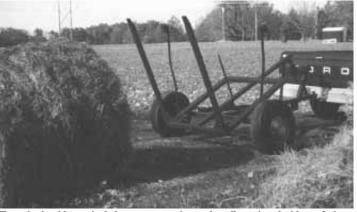
Two-wheel caddy carries bale on a rectangular steel cradle equipped with two forks at bottom and a removeable spear in middle. It can be pulled behind a pickup or mounted on a tractor 3-pt. hitch.
