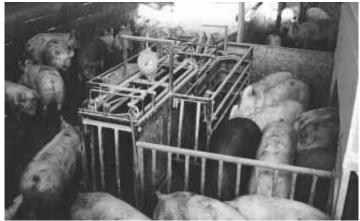
Built out of 1-in. sq. tubing, sorter features a swinging paddle that automatically closes behind hog once he enters weigh scale so it's set for the next hog and prevents the first one from backing out.
