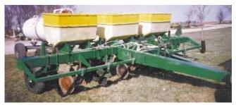
Kirk used a 6-row Deere planter toolbar and Deere dry fertilizer attachment to build rig. Lets him apply dry fertilizer and anhydrous ammonia at same time.
