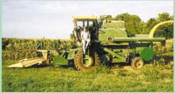
Stoll equipped his Deere 4420 combine with parts from a Deere pull-type forage harvester, mounting the harvester's header on front and the auger and blower on back. Lets him shell corn conventionally and chop silage into a wagon at the same time. grazing. That also reduces the need for hay. leaves.
