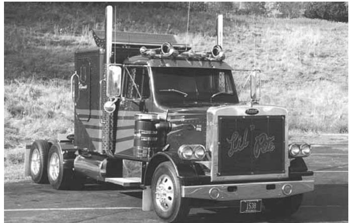
Mini-semi is powered by a Detroit 453T 4-cyl. turbocharged 190 hp diesel engine. It has a Fuller 9-speed transmission.
